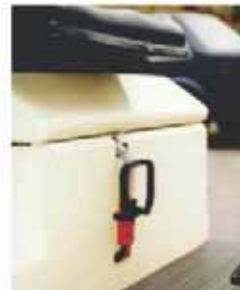
Emergency stop switch by disconnect the battery connector.
